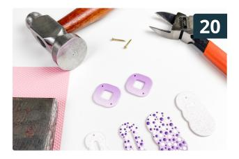
To join the pieces, use a rivet. Gather round headed nails, pliers, a hammer and an anvil or similar surface.
