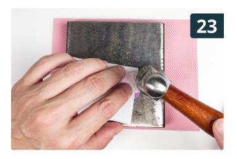
Place the pieces face down on the anvil and gently hammer the nail until it flattens and covers the hole, securing the pieces together. You can protect the clay with sheets of paper to avoid marks.
