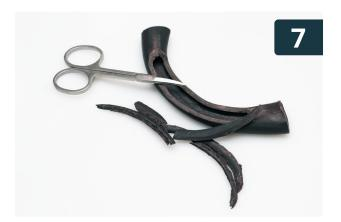
After the cylinder cools down, use fine scissors to cut out a center channel from the front part of the cylinder.
